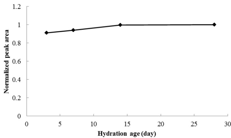
Fig. 5.7. Evolution of peak area for calcium hydroxide in the cement paste hydrated for 3 to 28 days
